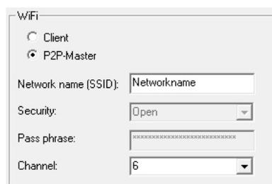
The screenshot shows a 'WiFi' configuration window. At the top, there are two radio buttons: 'Client' and 'P2P-Master' (which is selected). Below this, there are four input fields: 'Network name (SSID):' with the text 'Networkname', 'Security:' with a dropdown menu showing 'Open', 'Pass phrase:' with a masked input field containing asterisks, and 'Channel:' with a dropdown menu showing '6'.
