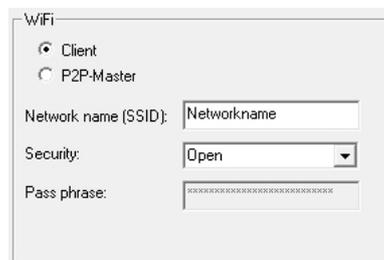
The screenshot shows a 'WiFi' configuration window. At the top, there are two radio buttons: 'Client' (which is selected) and 'P2P-Master'. Below this, there are three input fields: 'Network name (SSID):' with the text 'Networkname', 'Security:' with a dropdown menu showing 'Open', and 'Pass phrase:' with a masked input field containing asterisks.
