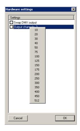
After confirmation with OK the interface will be configured accordingly and the settings will be saved permanently. The settings will be stored after turning off and can be changed only with a renewed configuration.
