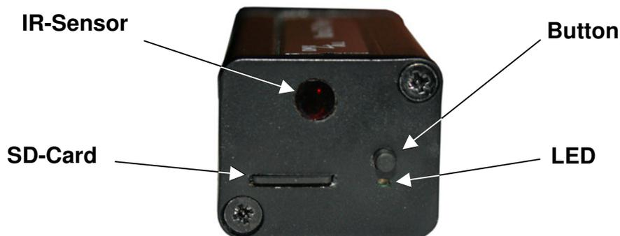
The **NanoSD Player** has a button as well as a LED to operate at the device.
