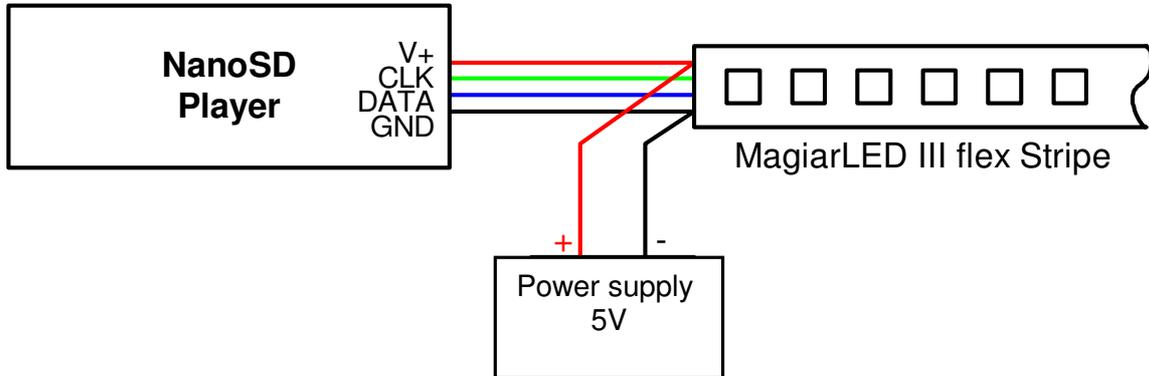
**Example for connecting Stripes with one controlling signal (DATA)**
