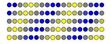
The Fade Moving Colors effect with a length equal to 0 controls all LED pixels equally. The colors are faded softly one after the other.
