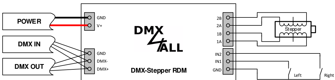
Connection with unipolar stepper motor
