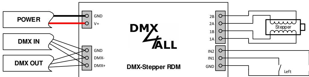
Connection with bipolar stepper motor
