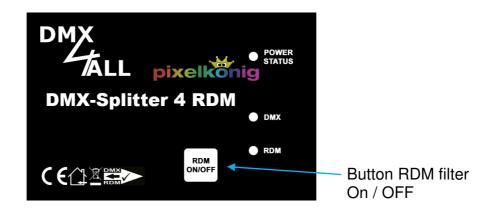
To turn on or off the RDM filter, the button RDM ON/OFF must be pressed for ca. 3 seconds.
