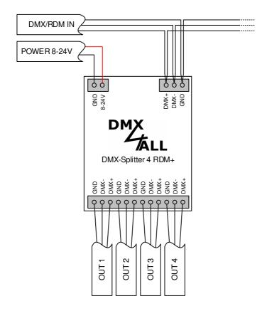
If more than 4 outputs are needed, several DMX-Splitter 4 RDM can be combined as follows:
