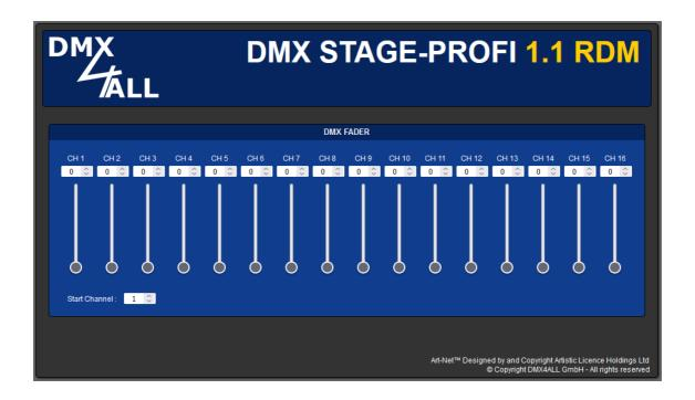
From the set start address (Start Channel) 16 sliders and entry fields for setting the DMX values can be used.
