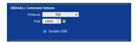
The control with the DMX4ALL commands can be made by sending RAW data packets via TCP or UDP to the set port.
