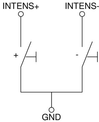
wiring with the UP/DOWN key
