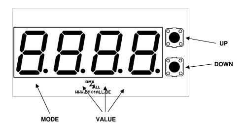
The adjusted operation mode MODE is displayed as R for Address-Mode and L for the ChannelAdd-Mode.
