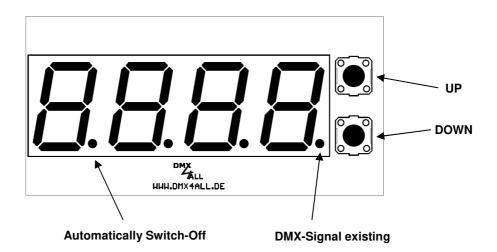
The activation of the automatically switch-off is signalled with a permanent lighting point. If the point is not lighting so the automatically switch-off is deactivated and the display doesn't shut down.
