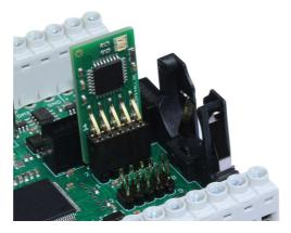
The DCF77 signal from the DCF77 sensor must be connected to IN8.
