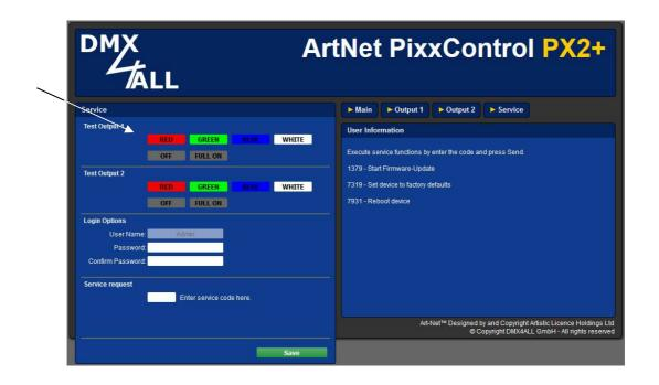
For the *Test Output* no control signal is to send to the ArtNet PixxControl PX2+! An external control signal always has priority over a test output.
