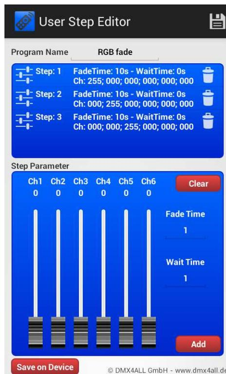
A list with all single steps will be shown. In each entry the Fade Time, Wait Time and the channel value is shown.
