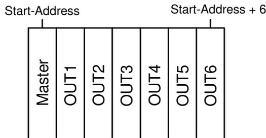
Is no Master-Dimmer activated the assignment is as follows:
