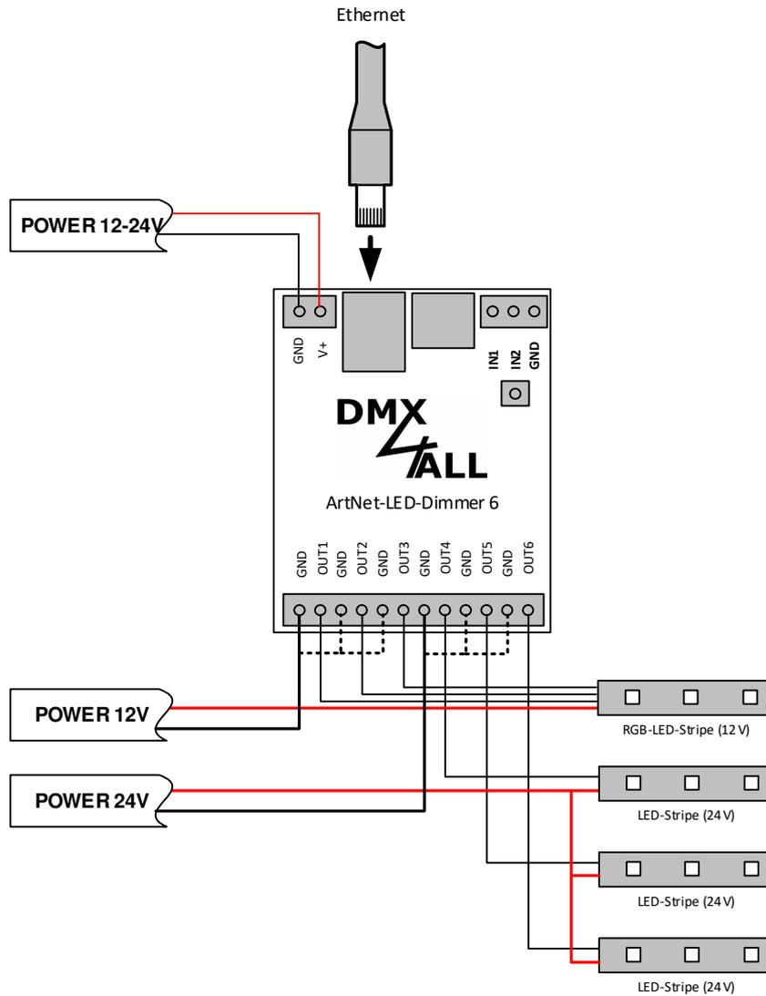
..... Connections according to the needed power for the LED-Stripes directly wired from power supply !
