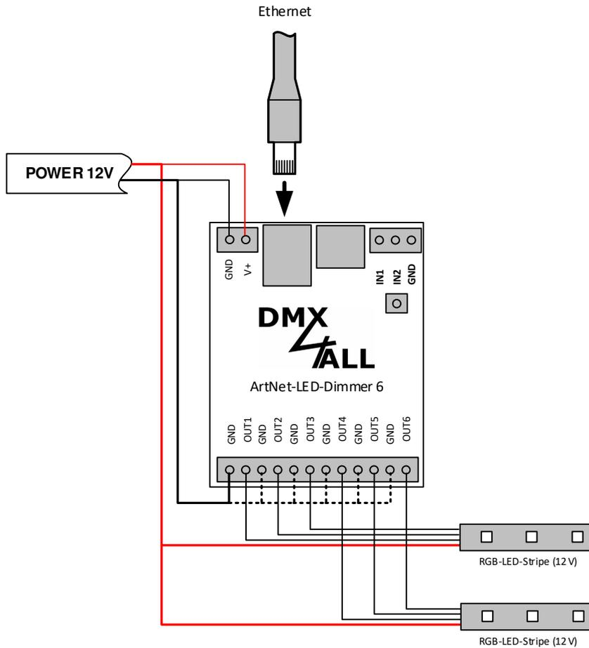
..... Connections according to the needed power for the LED-Stripes directly wired from power supply !
