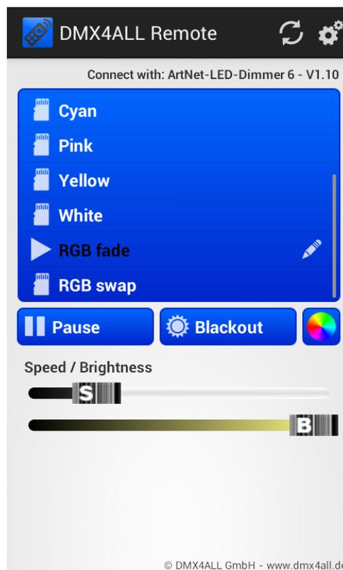
By tipping a programs name within the list the according program will be run via the ArtNet-LED-Dimmer. The executed program is marked with a symbol ▶.
