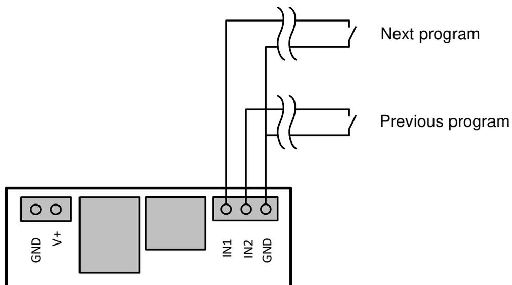
If a button is connected between IN2 and GND, it can be used to select the color changes / programs in reverse order (User 10 > User 1).
