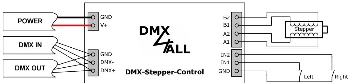
Connection with bipolar stepper motor
