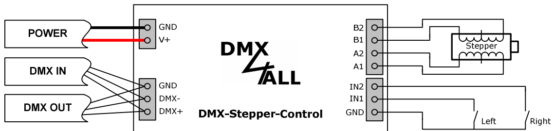
Connection with unipolar stepper motor
