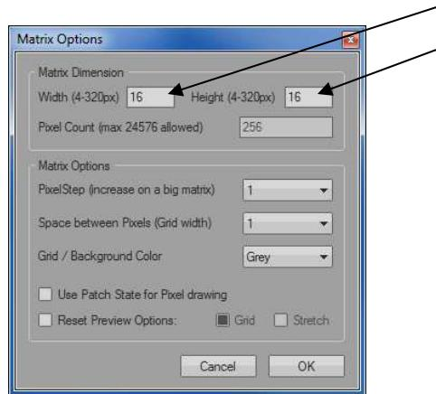
Here the width and height for the LED-Surface is adjustable.
