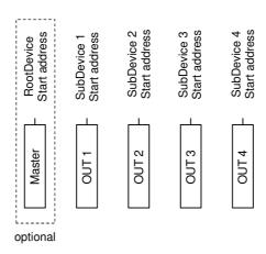
The assignment of the DMX addresses in SubDevice mode is as follows:
