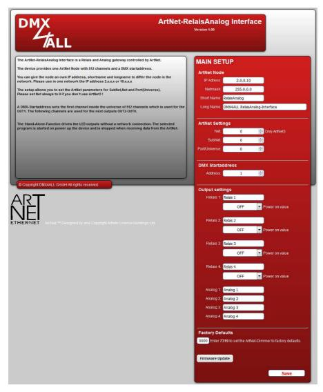
Each ArtNet-Node needs an own **IP-Address**, so the assignment in the network is clear. Use in accordance to the ArtNet-Specification the IP-Address 2.x.x.x or 10.x.x.x.
