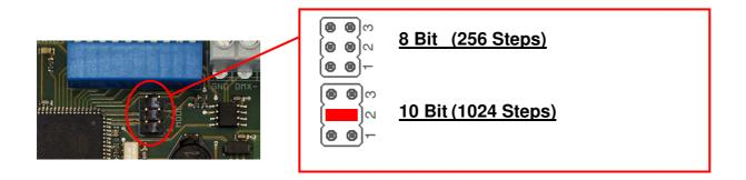
Depending on the resolutions setting the analog output there is needed per output one or two DMX-channels, as shown in the following picture.
