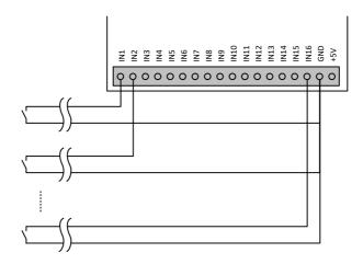
For the LONG DISTANCE inputs, we recommend cable lengths not exceeding 25m. Depending on the environment and cable type, longer distances may be possible.
