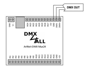
At the DMX-Output a DMX-Signal with 512 DMX-Channels will be outputted. With the "DMX Output Mode" (setting in the web interface) the following DMX output properties can be selected:
