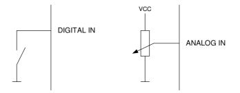
Some of the pins of the DMX710 can be used as digital or analog inputs. In the digital mode you have to connect a switch to GND. The analoge mode permit a signal from GND to VCC.
