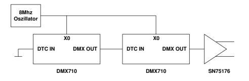
The DMX710 is cascadeable, as the DMX exit is connected with the DTC entrance of the next component. The last DMX exit goes to a line driver. It is possible to use one oszillator for all DMX710.
