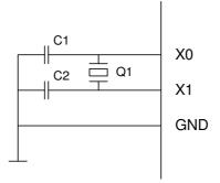
This example illustrates how to use the DMX710 with a 8MHz crystal. The value of the capacitors should be in the range of 12-33pF.
