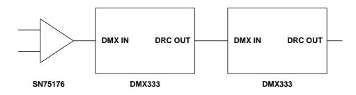
The DMX333 is cascadeable, as the DRC exit is connected with the DMX entrance of the next component. The first DMX input receives the signalfron the line driver.
