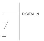
Some of the pins of the DMX333 used as digital inputs. This pins are connected with a switch to GND.
