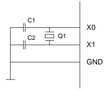
This example illustrates how to use the DMX333 with a 8MHz crystal. The value of the capacitors should be in the range of 12-33pF.
